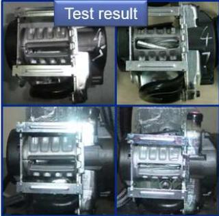
The frame took place fracture when pulling force reached 20kN as similar test result of 17-19kN.
