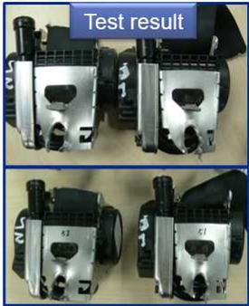
The frame took place fracture when pulling force reached 16kN as similar test result of 16-18kN.
