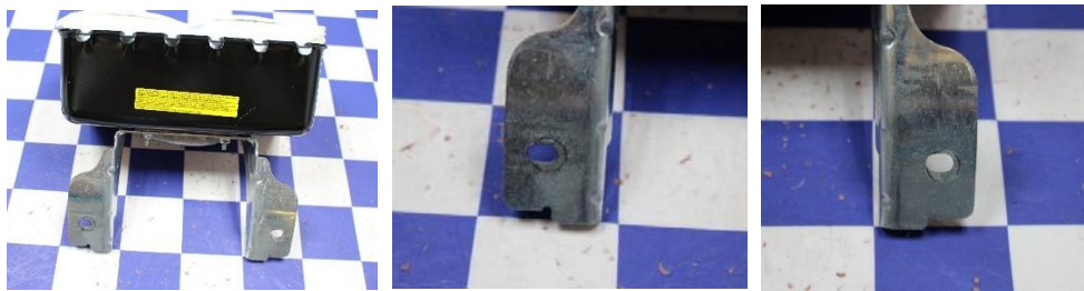
Figure 8 - PAB Modules after Test
